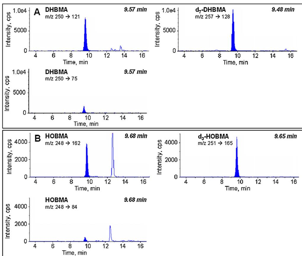
**Fig. 3.** Chromatogram of a spiked non-smokers urine sample showing the mass transitions of the analytes and internal standards of the analyte group 1. Determined analyte levels were: 180  $\mu\text{g/L}$  of DHBMA (A) and 183  $\mu\text{g/L}$  of HOBMA (B).
