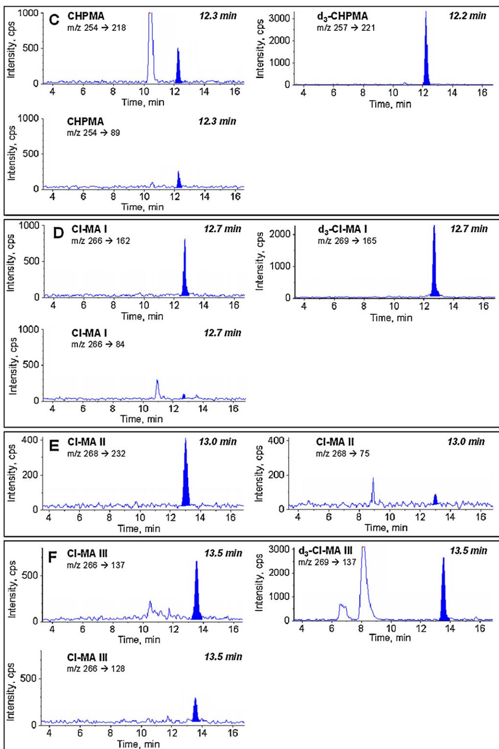
**Fig. 4.** Chromatogram of a spiked non-smokers urine sample showing the mass transitions of the analytes and internal standards of the analyte group 2. Determined analyte levels were: 26.5  $\mu\text{g/L}$  of CHPMA (C), 30.4  $\mu\text{g/L}$  of CI-MA-I (D), 50.7  $\mu\text{g/L}$  of CI-MA-II (E) and 23.6  $\mu\text{g/L}$  of CI-MA-III (F).
